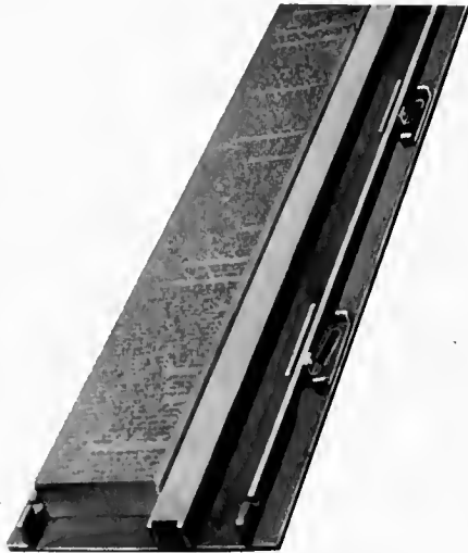
Illustrating the end-piece removed, with guide bar in position, the type appearing just as the caster would deliver it on to the galley.
